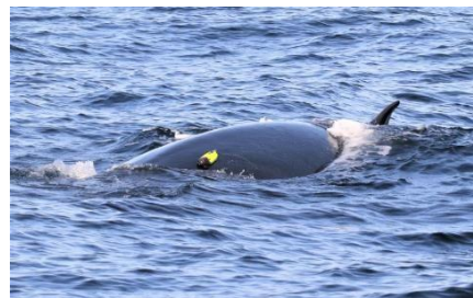
Fig 15: An Acousonde TM tag attached to whale via suction cups (Source: NOAA Fisheries/MMPA Permit)
